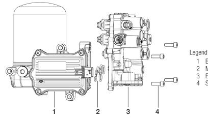
1 EAC2.1 Air Dryer 2 Moulded seal
