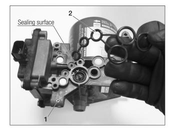
Position the EAC2.1Multi protection Valve (3) to EAC2.1 Air Dryer Unit (1).
