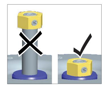
For spring brakes with the built-in release device, using a 24 mm spanner rotate the hexagon nut clockwise a minimum of 50 turns. The red indicator must be completely embedded in the hexagon nut.
