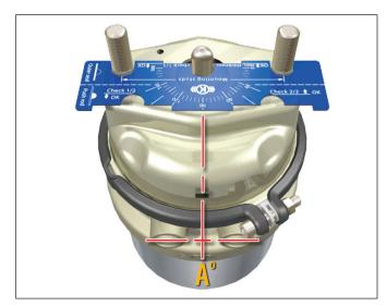
measure the angle (B) of the 'ears' of the clamp ring
