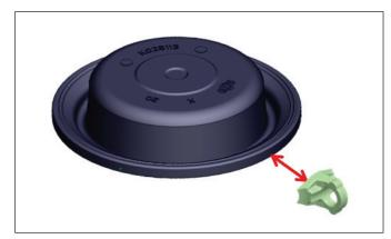
Check that the quad-ring seal is correctly located in the non-pressure plate by using the Knorr-Bremse Maintenance Gauge to check the seal height.
