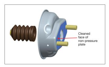
Use an appropriate tool (with no sharp edges) to locate the bellows in the non-pressure plate, avoiding any damage to the quad-ring seal of the bellows.
