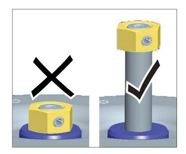
For spring brakes with the built-in release device, the red indicator must protrude through the hexagon nut by approximately 8 mm.
