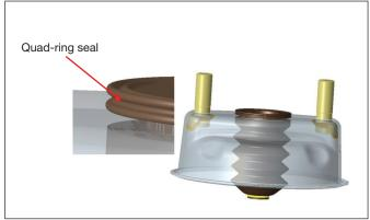
Grease the internal diameter of the rubber boot which is in contact with the push rod of the push rod/push plate assembly. Use Fuchs "Renolit" HLT2 grease (Part No. II14525 included in Knorr-Bremse service kits) or an equivalent.
