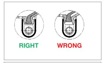
Fit the clamp ring ensuring correct alignment all around and take care to ensure that the original angular position of the ports and clamp rings ears are maintained. Use the Knorr-Bremse Maintenance Gauge to check this.
