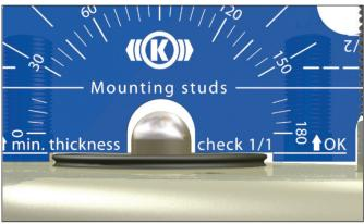
Check that the push plate is correctly located in the diaphragm by using the Knorr-Bremse Maintenance Gauge to check the push rod protrusion.
