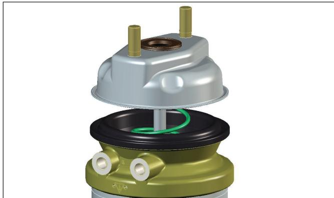
Press the non-pressure plate onto the intermediate flange with the diaphragm between these two parts by maintaining a maximum load of 6000 N.
