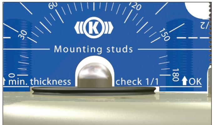
Check that the push plate is correctly located in the diaphragm by using the Knorr-Bremse Maintenance Gauge to check the push rod protrusion.
