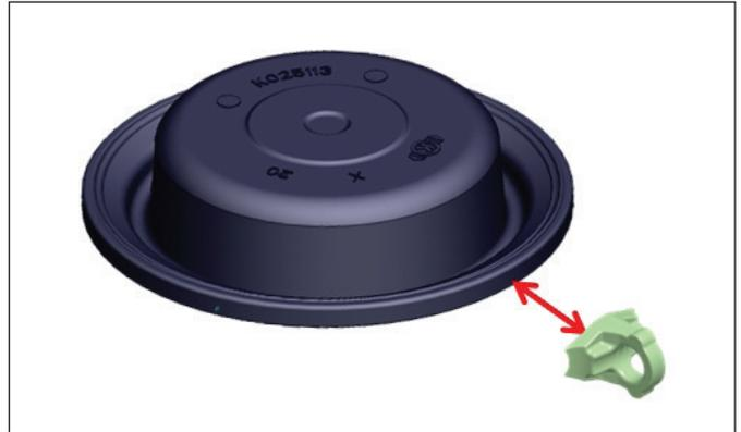
Check that the quad-ring seal is correctly located in the non-pressure plate by using the Knorr-Bremse Maintenance Gauge to check the seal height.
